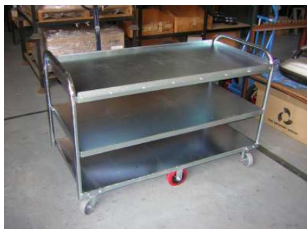
Special 'E' type fitted with lips to edge of tray and 6 castor set up
